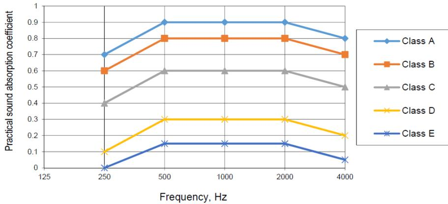
Figure 3.1: The reference curves limiting the different sound absorption classes.
